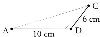
$$\begin{aligned} AC &= \sqrt{10^2 + 6^2} \\ &= \sqrt{136} \end{aligned}$$
