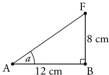
$$\begin{aligned}\tan \alpha &= \frac{\text{Opposite}}{\text{Adjacent}} = \frac{8}{12} \\ \alpha &= \tan^{-1}\left(\frac{2}{3}\right) \\ &= 33.690^\circ \text{ (or } 0.588 \text{ radians) (to 3 d.p.)}.\end{aligned}$$
