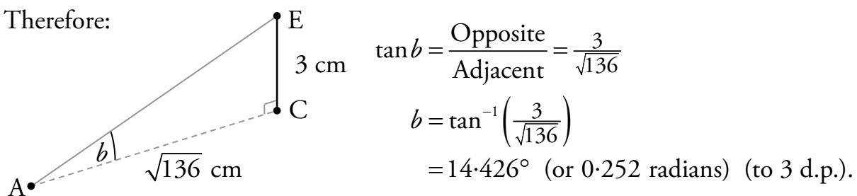
$$\begin{aligned} \tan b &= \frac{\text{Opposite}}{\text{Adjacent}} = \frac{3}{\sqrt{136}} \\ b &= \tan^{-1}\left(\frac{3}{\sqrt{136}}\right) \\ &= 14.426^\circ \text{ (or } 0.252 \text{ radians) (to 3 d.p.)} \end{aligned}$$
