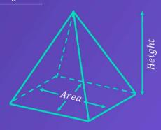
To calculate the volume of a pyramid, multiply the area of its base by its height and divide by three.
