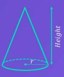
To calculate the volume of a cone, multiply its height by its radius squared and by pi then divide by three.
